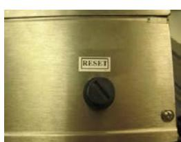
With the unit unplugged and fully cooled off, unscrew the know to expose red button
